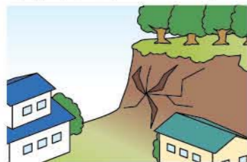
Cracks form on slopes.
